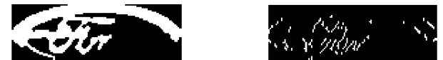
Figure 8. Third candidate for the license plate (left) and detected vertical edges (right)
