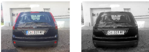
Figure 2. Original vehicle image (left) and the result of the preprocessing algorithm (right)
