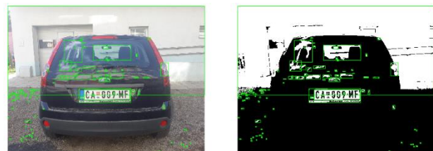
Figure 3. All found regions in the digital image on the original RGB image (left) and on the binarized image (right)
