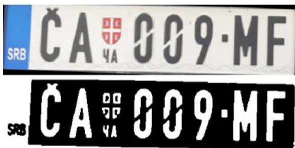
Figure 18. Original license plate image (top) and the result of the preprocessing (bottom)
