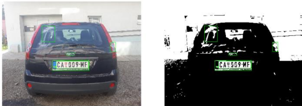
Figure 4. Remaining regions after discarding regions with non-negative Euler number, original RGB image (left) and the binarized image (right)
