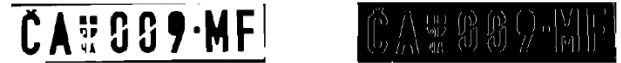
Figure 7. Second candidate for the license plate (left) and detected vertical edges (right)
